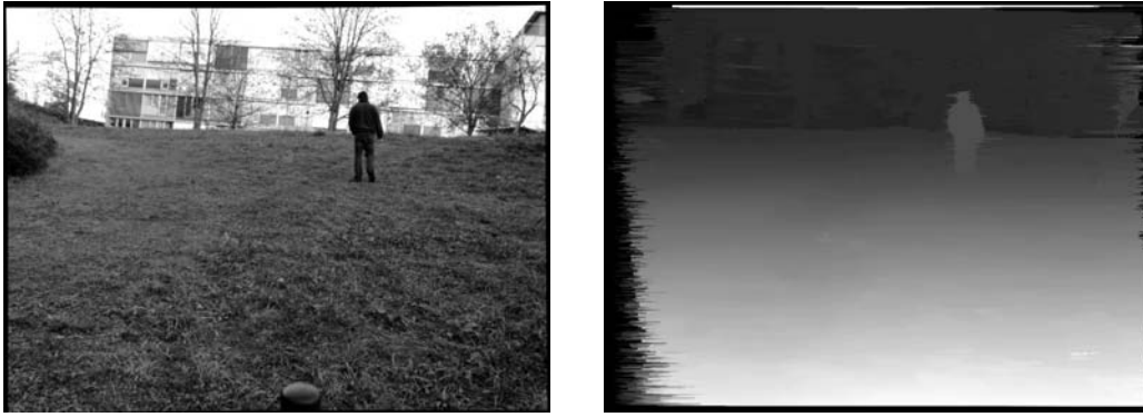
Figure 5.17: Undistorted left image and resulting disparity map
