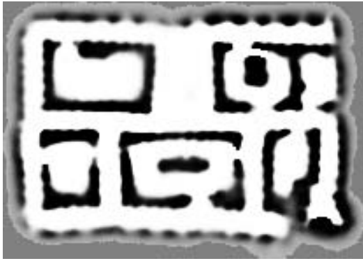
Figure 3.1: Occupancy grid map [Thrun 96b] Each pixel represents one grid cell, darker colors indicate higher occupancy probabilities. Thus, white pixels denote free space, gray pixels represent unknown areas and black pixels stand for obstacles.
