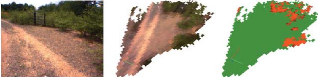
Figure 6.6: Learning from proprioception (LfP) The figure shows a sample image, a projection onto the local map and learned traversability predictions (Source: [Howard 06])
