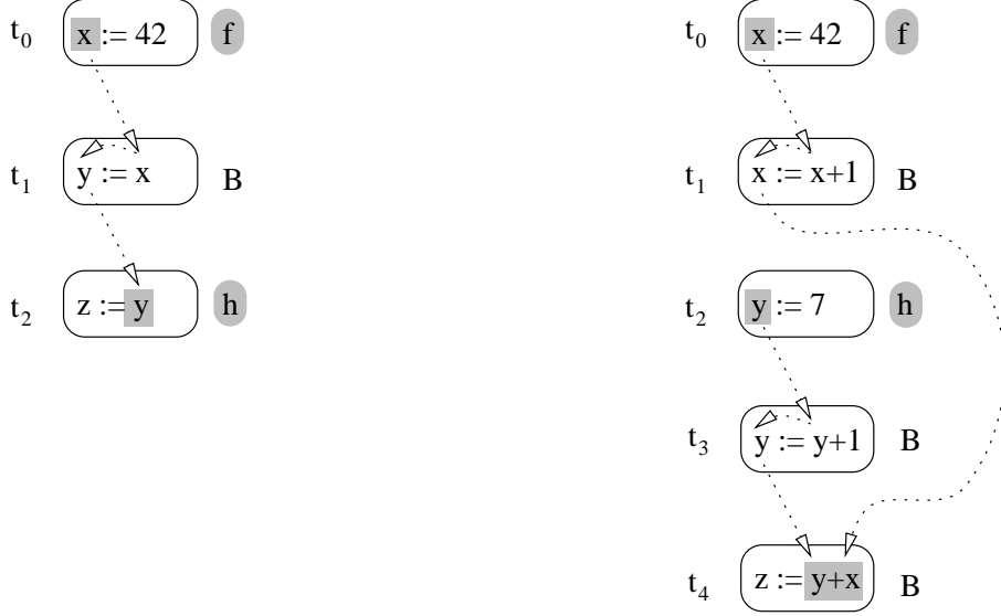
Figure 12: Two examples of indirect data dependences.
