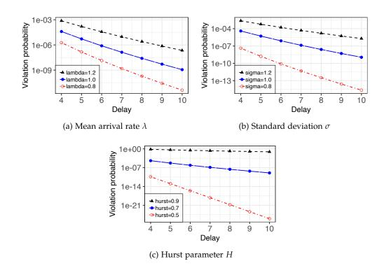
Figure 4.7: Parameter sensitivity of fractional Brownian motion on the delay bounds using PMOO (sink tree).
