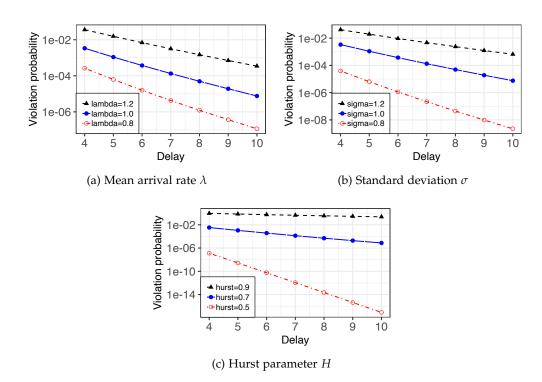
Figure B.3: Parameter sensitivity of fractional Brownian motion on the delay bounds (tandem queue).
