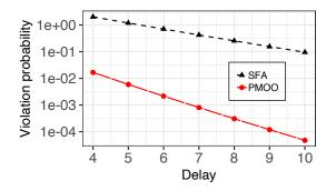
Figure B.2: Comparison between delay violation probabilities using SFA and PMOO (tandem queue).
