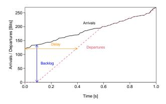
Figure 2.2: Backlog and virtual delay for an arbitrary arrival and departure process.
