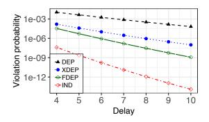
Figure 4.10: Delay bound comparison for three servers with increasing degree of dependence.
