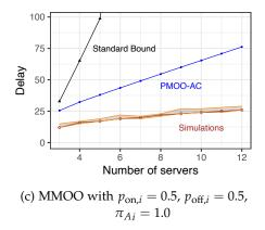
Figure 5.7: Stochastic delay bounds for the extended overlapping tandem under constant rate servers with rates  $C_i = 2.0$  for i = 1, ..., 13.
