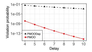
Figure 4.9: Comparison between delay violation probabilities for independent and dependent cross-flows using PMOO (sink tree).
