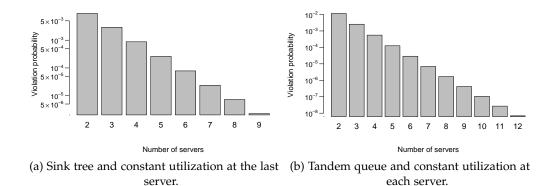
Figure 4.8: Delay violation probability for different lengths using PMOO.
