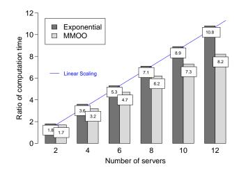
Figure 7.7: Computation time comparison for the state-of-the-art and power-mitigator approach.
