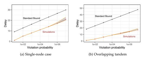
Figure 5.2: Stochastic delay bounds: Simulation results and SNC bounds (for traffic with exponentially distributed increments and constant rate servers). For more details, see Section 5.3.
