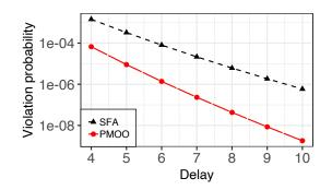
Figure 4.6: Comparison between delay violation probabilities using SFA and PMOO (sink tree).
