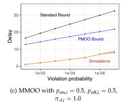
Figure 5.9: Stochastic delay bounds and simulation results for the tree network with constant rate servers and rates  $C_i = 2.0, i = 1, ..., 4$ .
