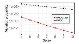
Figure B.4: Comparison between delay violation probabilities for independent and dependent cross-flows using PMOO (tandem queue).
