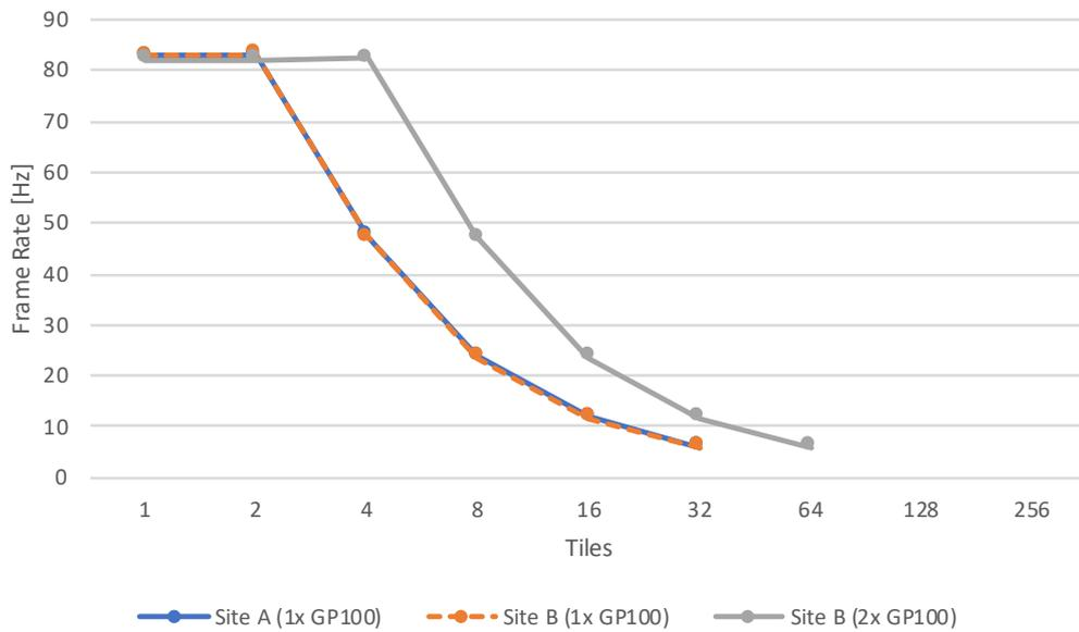
**Fig. 6.10:** Weak scaling (N:1): Client-side achieved frame rate for streaming full 4K frames of *Ice* sequence to Site A (blue) and Site B (orange, gray) using H.264 at 32 Mbps.
