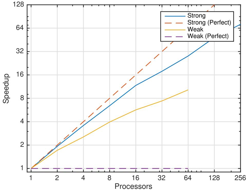
**Fig. 4.8:** Strong and weak scaling behavior of the distributed layered depth image rendering approach using HPX on the *Elwetritsch* cluster. Subblocks of the *jet5 velocity* data set are distributed across nodes and rendered in parallel. The resulting partial images are composited to a single layered depth image afterwards. We achieve overall good strong scaling and excellent weak scaling characteristics.
