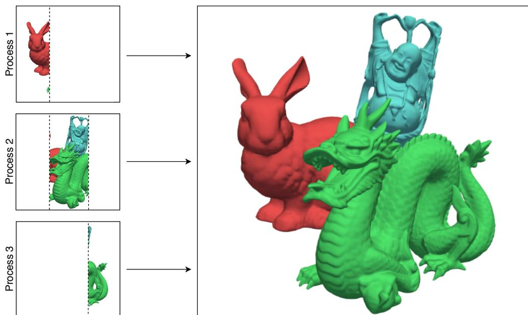
**Fig. 2.5:** Sort-first compositing. Every node has the complete data, but renders only a partial tile of the final image.
