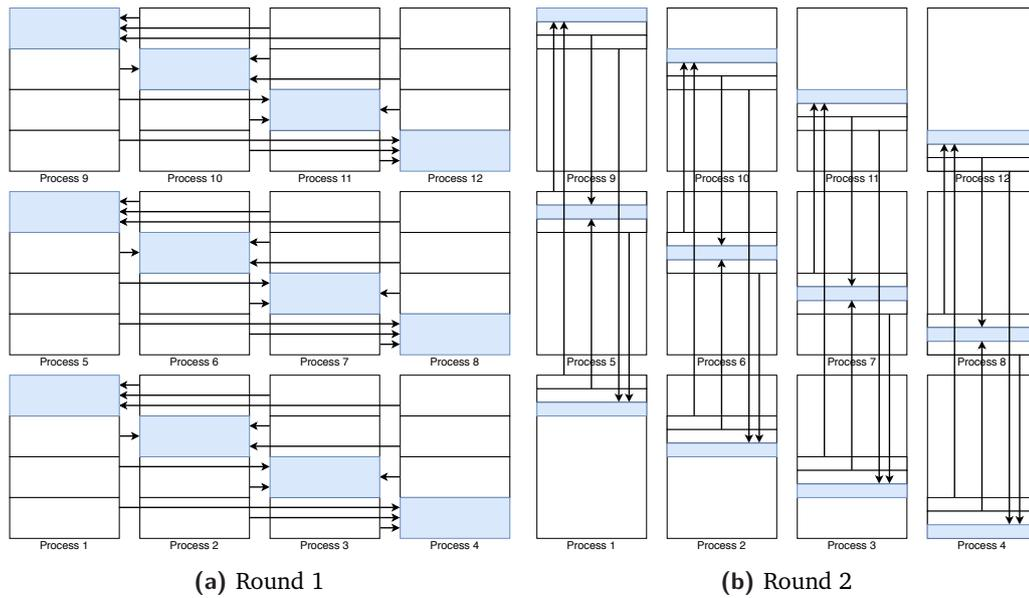
**Fig. 2.10:** Radix- $k$  compositing using twelve processes over two rounds with  $k = [4, 3]$ .
