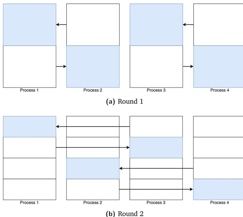
**Fig. 2.8:** Binary-swap compositing using four processes over two rounds. In each round the distance is doubled and the image size is halved.
