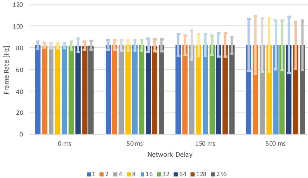
**Fig. 6.8:** Weak scaling (N:N) within Piz Daint: Mean frame rates and min/max ranges for different simulated network delays (+ 10% jitter), streaming up to 256 concurrent full 4K tiles of *Ice* sequence using H.264 at 32 Mbps.
