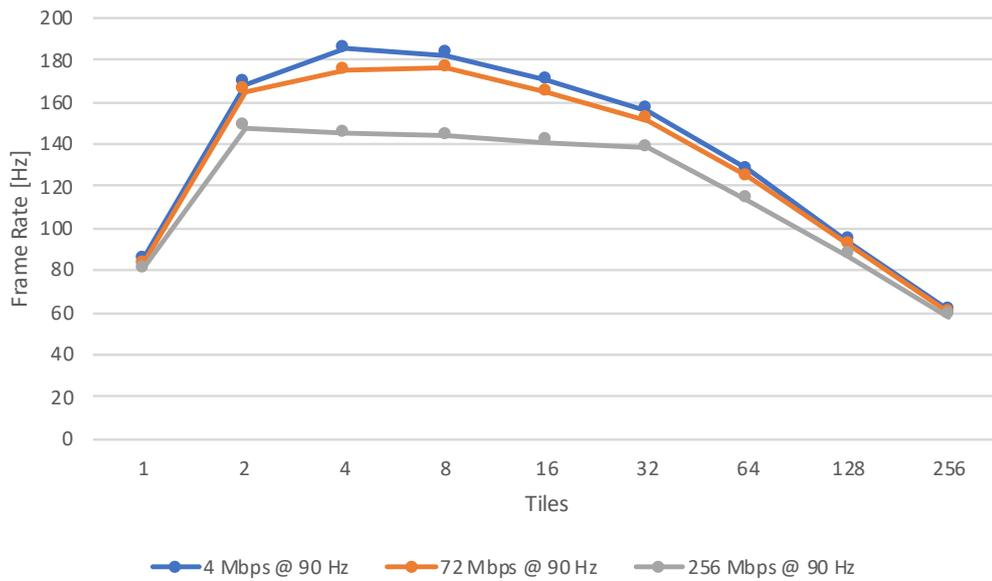
**Fig. 6.14:** Client-side frame rate for strong-scaled streaming of *Ice* 4K frames from up to 256 servers at different H.264 bitrates. Highest setting is limited by link bandwidth (gray).
