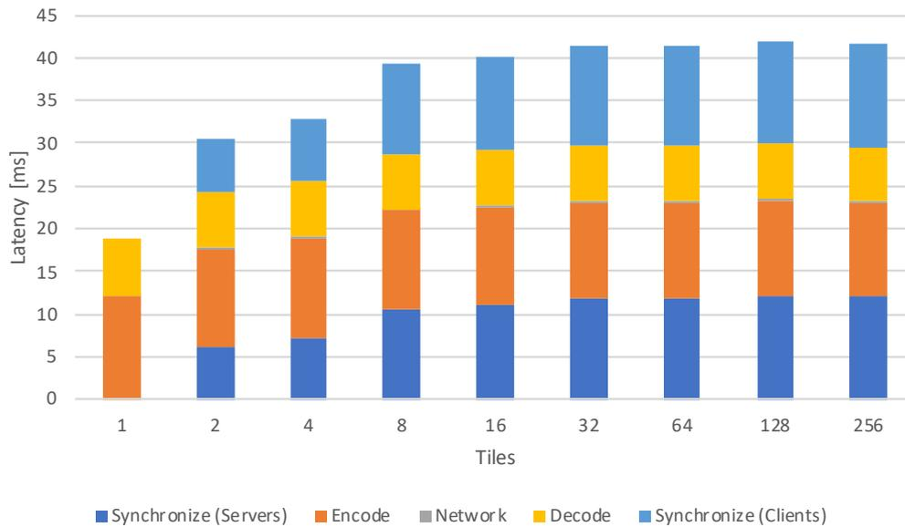
**Fig. 6.9:** Weak scaling (N:N) within Piz Daint: Pipeline latencies for full 4K streams of *Ice* using H.264 (32 Mbps).
