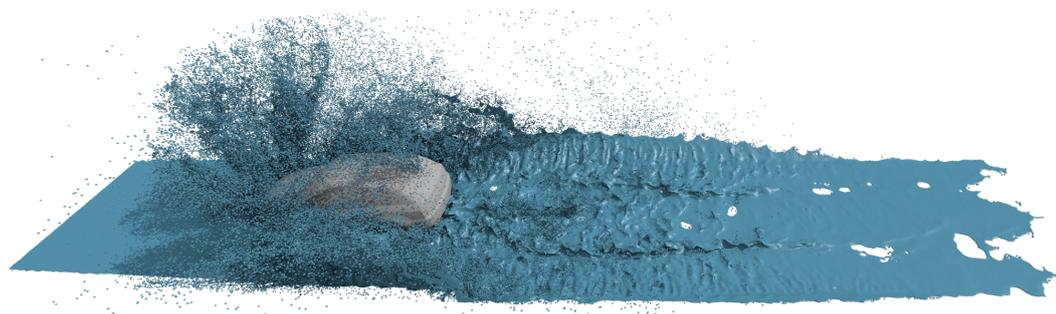
**Fig. 3.1:** Watercrossing simulation using 2.1 million particles. Rendered at 4K resolution with ambient occlusion and hard shadows in 2.4 seconds on 32 Xeon Phi KNL nodes of the Stampede2 supercomputer.
