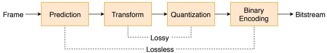
**Fig. 2.12:** Encoding pipeline for the H.264/H.265 video codec family consisting of both lossless and lossy compression steps.
