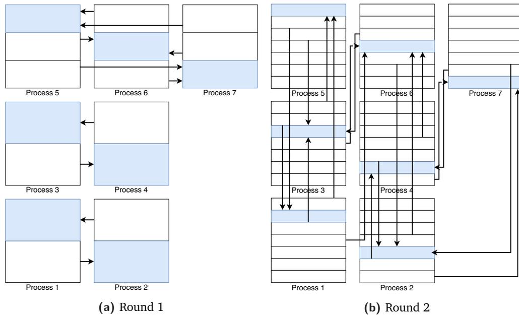
**Fig. 2.9:** 2-3-swap compositing using seven processes. In the first round (left), groups of twos and threes execute direct send compositing. In the second round (right), each process owns 1/7 of image, where the group size in the second round is between two and five.
