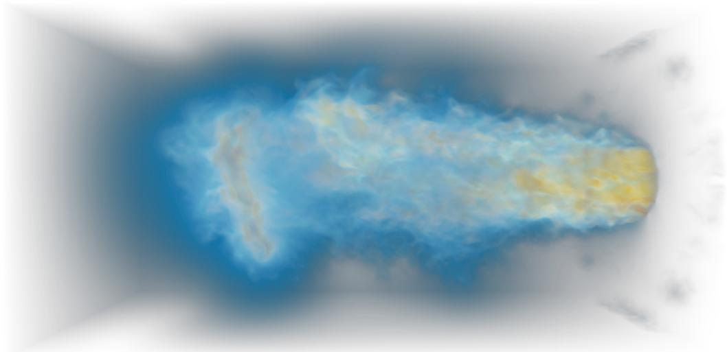
**Fig. 5.1:** The *jet* reference data set used for all benchmarks with  $2048^3$  voxels (32 GB) on a single node. For weak scaling, the number of voxels is increased proportionally to the number of cores, up to  $6502^3$  (275 gigavoxels) on 32 nodes. All renderings are performed at  $3840 \times 2160$  resolution.
