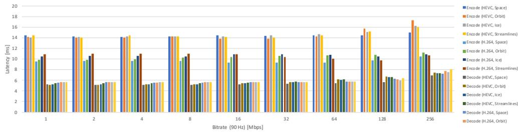
**Fig. 6.4:** Comparison of en-/decode latencies for the four test scenes at different bitrates for H.264 and HEVC at 4K resolution.
