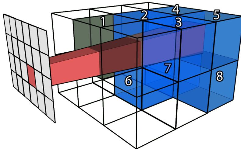
**Fig. 5.2:** Hybrid parallelization in both image and data space. For each tile, the set of visible blocks is topologically sorted and composited using a distributed binary tree communication scheme. The numbering represents an arbitrary enumeration of the visible blocks within the highlighted tile's frustum. See Figure 5.3 for the corresponding compositing tree. Note that block 1 is discarded due to empty-block skipping.
