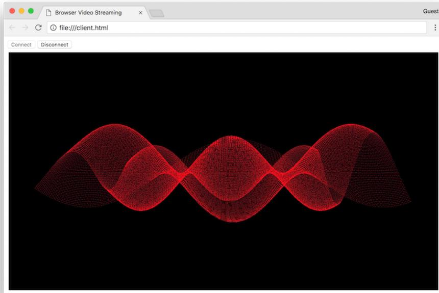
**Fig. 6.16:** Streaming unmodified CUDA *simpleGL* example from headless node to web browser using EGL-based shim library as GLUT replacement, WebSocket-based bidirectional communication (including interaction), on-the-fly MP4 wrapping of raw H.264 stream, and a JavaScript client.
