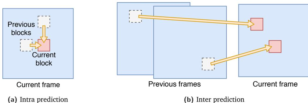
**Fig. 2.13:** Prediction leverages the redundancies between spatially and temporally neighboring pixels. While intra prediction only considers previously encoded blocks from within the same frame, inter prediction also utilizes blocks from previously encoded frames.
