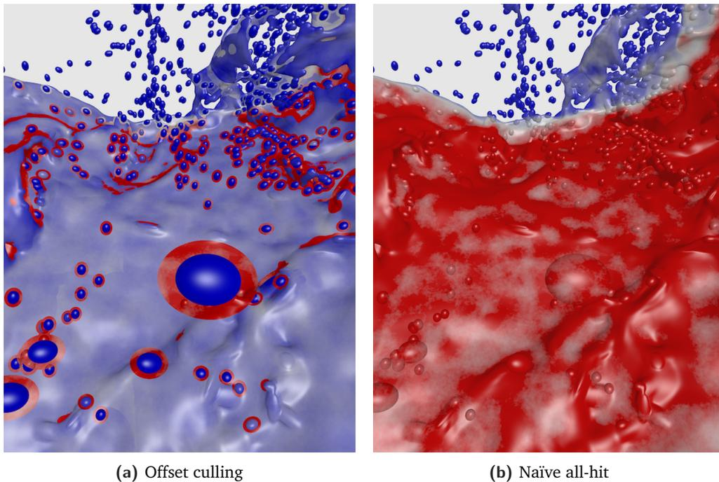
**Fig. 3.4:** Total number of ellipsoids collected per ray, from zero (blue) to 200 (red). Using offset culling dramatically reduces the number of smoothing kernels considered for surface sampling. Red halos in Figure 3.4a indicate areas where the frontmost kernels are hit, but the surface threshold is not reached and offset culling terminates. Thus, an all-hit intersection is performed to reach the real surface intersection.
