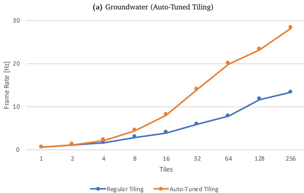
**Fig. 6.15:** Left: *Groundwater* scene used in the OptiX-based pathtracer for the 4K strong scaling rendering experiments with auto-tuned distribution of tile sizes. Data courtesy of TACC/FIU. Right: Client-side frame rate achieved for strong scaling of path traced image at 4K resolution on up to 256 nodes using fixed tile distribution (blue) and auto-tuned tile sizes (orange).
