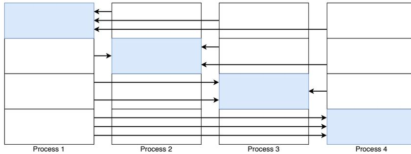
**Fig. 2.7:** Direct-send compositing using four processes. Each process is responsible for  $1/4$  of the final image.
