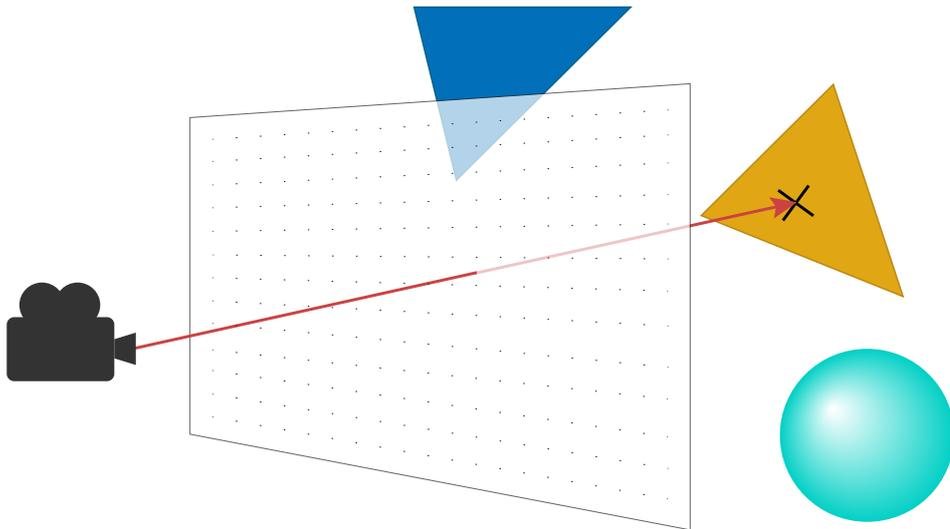
**Fig. 2.1:** In ray casting-based algorithms, e.g., ray tracing or direct volume rendering, rays are sent from the virtual camera, through each pixel of the screen and intersected with the scene.
