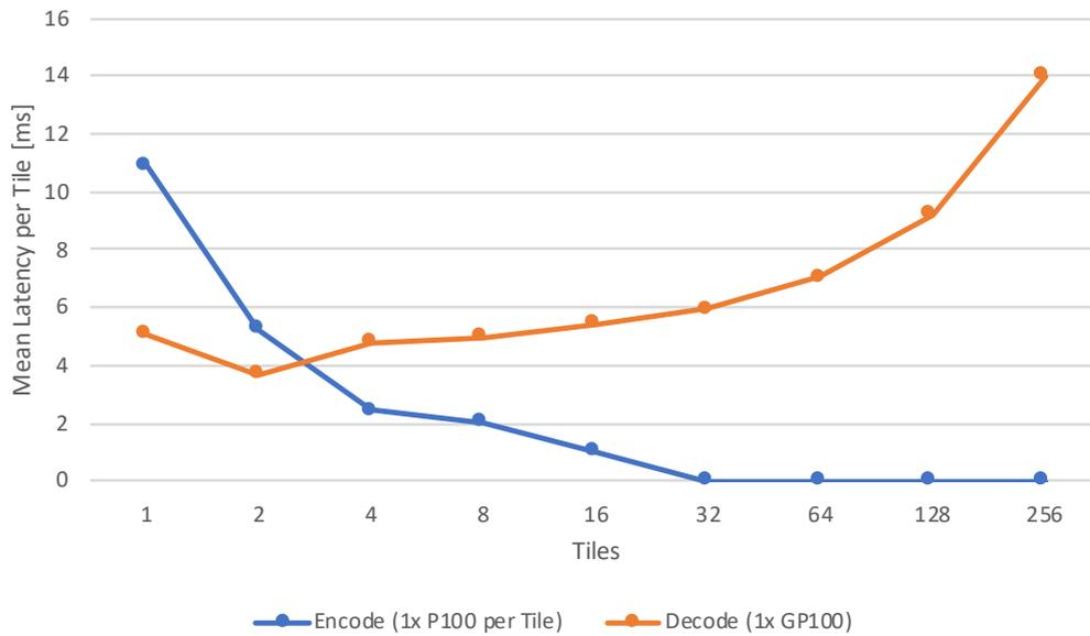
**Fig. 6.13:** Mean latency for encoding a 4K frame (blue) on the server side (strong-scaled, N:1) and decoding all tiles on the client side (Site B, orange) using H.264 (32 Mbps).
