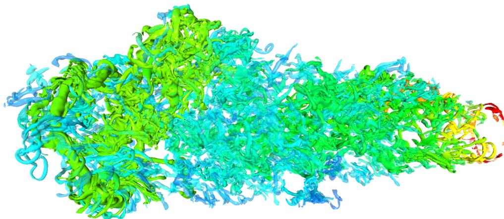
Fig. 4.1: Automatic segmentation of the turbulent jet5  $\lambda_2$  data set into 1024 branches based on branch persistence.
