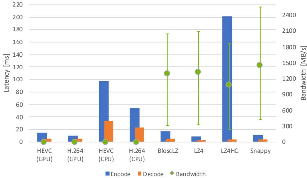
**Fig. 6.6:** Comparison of average en-/decode latencies and required bandwidths at 90 Hz for 4K using different GPU and CPU codecs. Bandwidth shows min/max ranges across test cases. H.264/HEVC configured to 32/16 Mbps at 90 Hz, others to maximum compression level.
