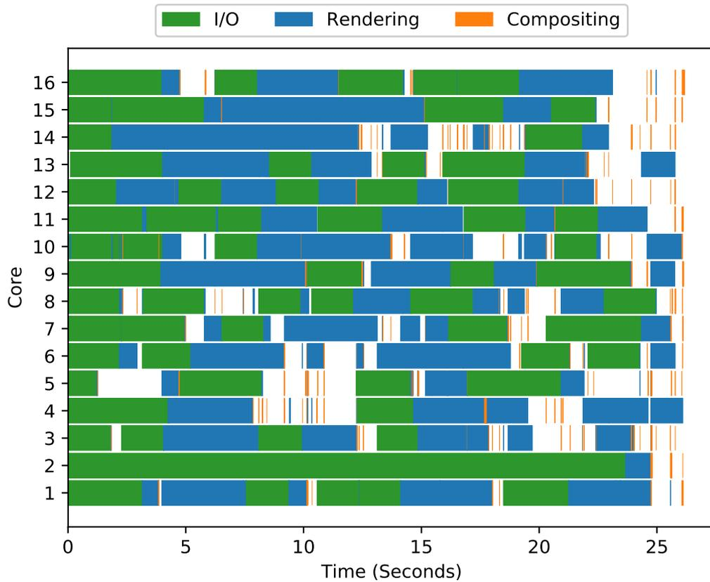
**Fig. 5.6:** Task scheduling for offline rendering of  $2048^3$  voxels using 16 cores on a single node at block size  $512^3$  and tile size  $960 \times 540$ . Block loading, rendering and compositing happen interleaved without barriers, so the resulting image is immediately ready after the final rendering and compositing tasks. Whitespace indicates unmet task dependencies such as outstanding I/O tasks or compositing partners.
