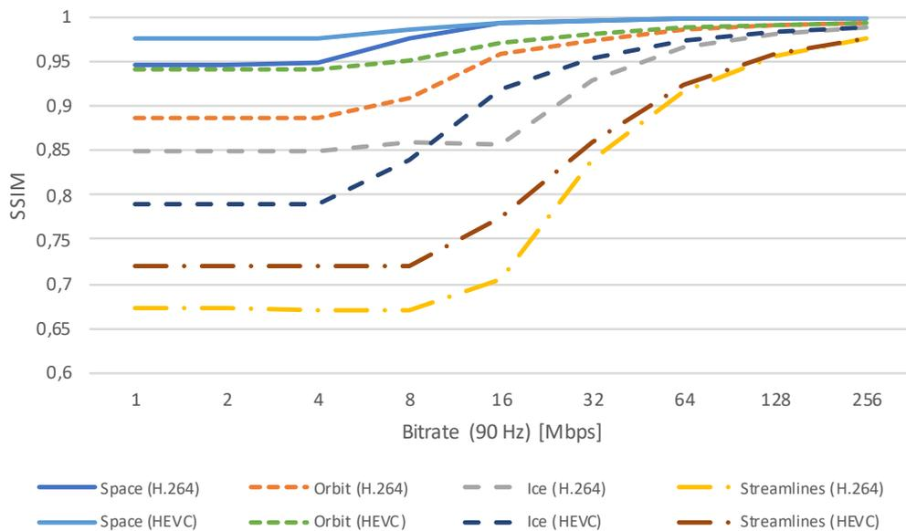
**Fig. 6.3:** Structural similarity (SSIM) index of the four test scenes at different encoder bitrates for H.264 and HEVC.
