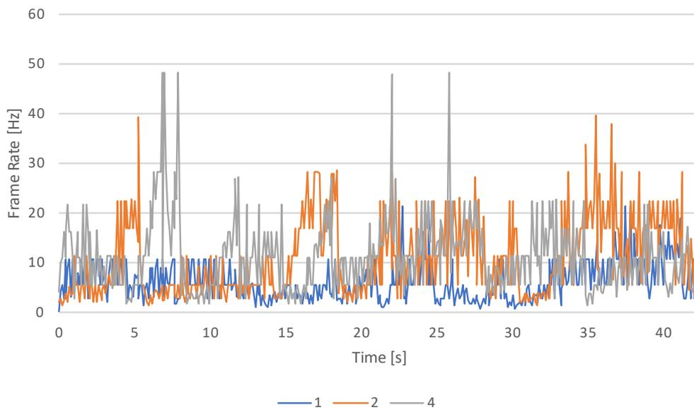
**Fig. 6.11:** Weak scaling (N:1): Streaming up to 4 full 4K frames of *Ice* sequence across Atlantic Ocean to Site C using HEVC at 16 Mbps. Frame rate sampled at 10 Hz.
