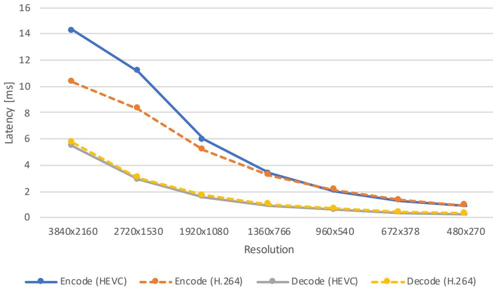
**Fig. 6.5:** Comparison of en-/decode latencies (averaged across test scenes) at different resolutions for H.264 and HEVC. Default bitrate for 4K at 90 Hz is 32/16 Mbps (H.264/HEVC), downscaled proportionally with pixel count.
