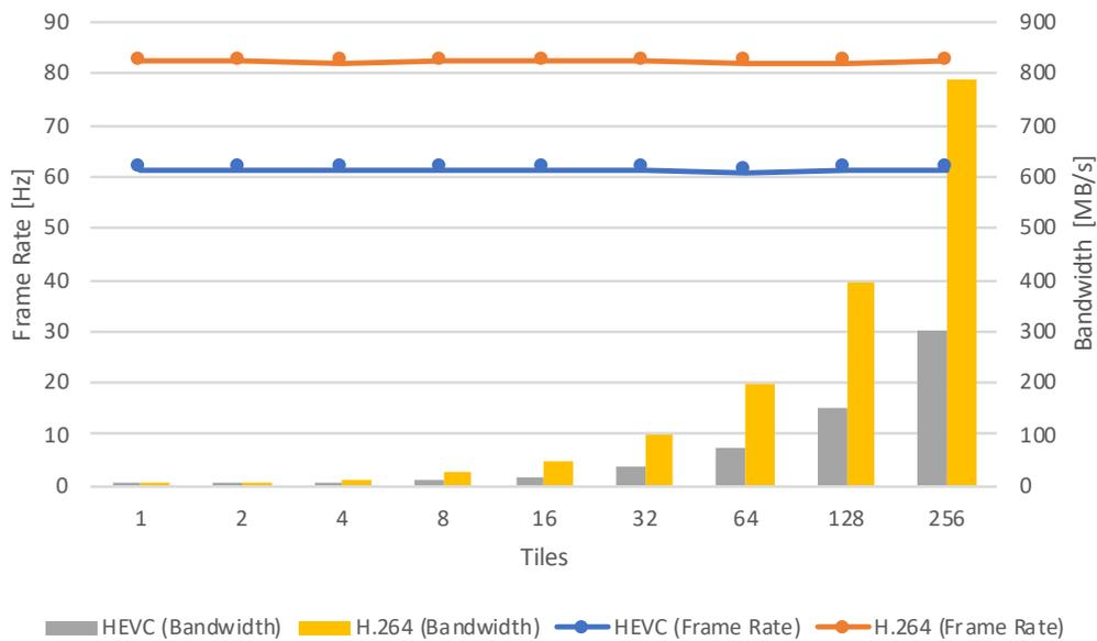
**Fig. 6.7:** Weak scaling (N:N) within Piz Daint: Client-side frame rates and bandwidths for up to 256 concurrent full 4K streams of the *Ice* video at 32/16 Mbps (H.264/HEVC).
