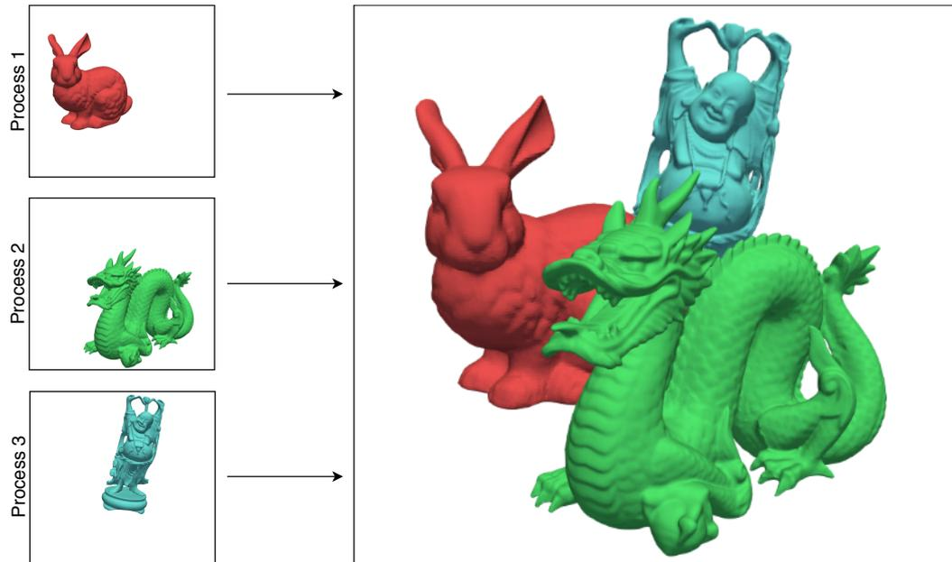
**Fig. 2.6:** Sort-last compositing. Every node renders a complete full-resolution image of a subset of the overall data.
