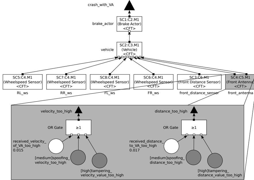
Fig. 2. CFT with security events of the ACC.
