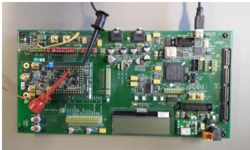
**Figure 5** 40nm test chip and board setup used for measurements to determine BER vs standby VDD.
