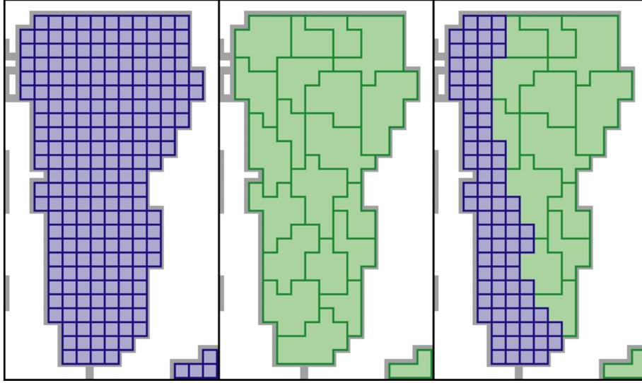
**Figure 3.** The different structures in the volume  $V$  consisting of the voxels (left) and the clusters (middle). An adaptive clustering (right) for  $V$  consists of small voxels in  $\mathcal{V}(\mathbf{x}^*)$  - here the left part of  $V$  - and large clusters elsewhere.
