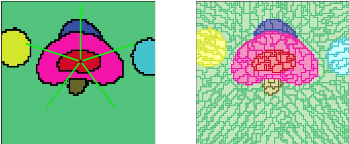
**Figure 17.** Left hand side: The organ geometry with boost and target (centre), the adjacent bladder (above target) and rectum (below target) and the two hips. The lines heading towards the isocentre (cross in the centre) visualize the beam directions. Right hand side: The clustering structure on level 3, which well represents the beam directions.
