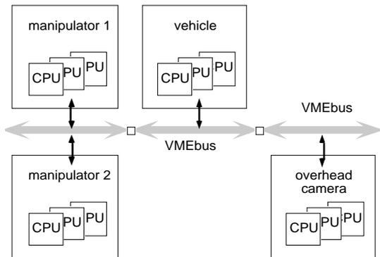
Fig. 2: Parallelism on the robot level: The autonomous mobile manipulation system KAMRO
