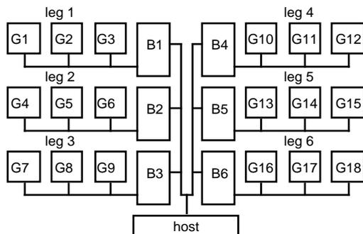
Fig. 3: Parallelism on the kinematics level: The 6-legged walking machine LAURON [17]
