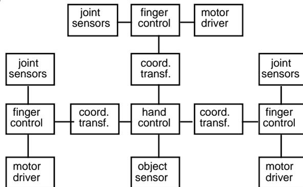
Fig. 4: Parallelism on the control level: The Karlsruhe Dextrous Hand [49]
