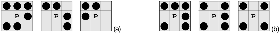
Fig.6: Examples for window settings; (a): p is not critical; (b): p is critical (probably dividing the region into two, three and four parts).
