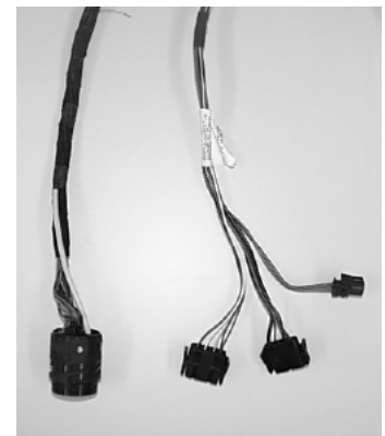
Figure 1: Section of the driver's door cable form for MERCEDES Class A (left) and Class C (right)
