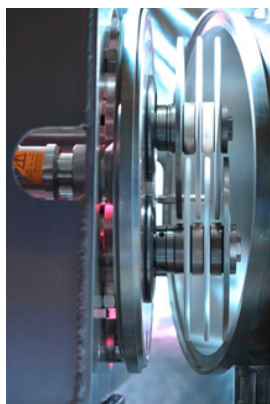
Figure 6. Arrangement of the filter disks in the DCF 152/0,14 filter [42].
