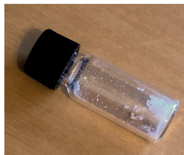
Figure 2. Purified, colorless, crystalline adipic acid that was obtained via catalytic oxygenation of cyclohexane.
