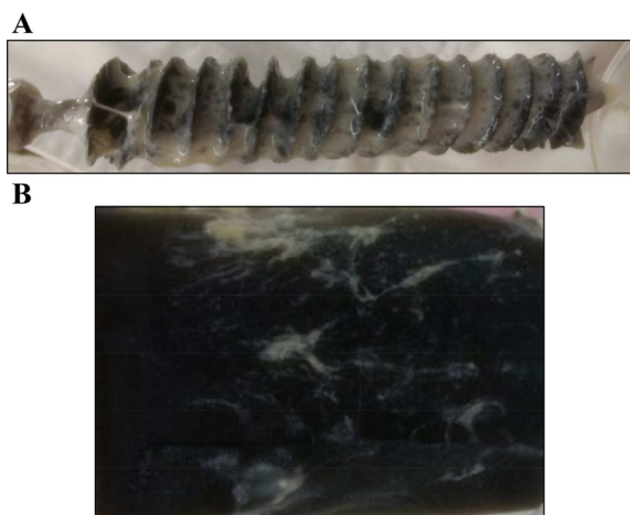
Figure 1. C. acetobutylicum biofilm formed on (A) the WE (length of the carbon brush: 110 mm, diameter of the brush: 21 mm) and (B) the CE after 48 h of an electro-fermentation at -600 mV in a single chamber bioelectrochemical reactor.
