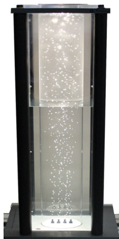
Fig. 3 Experimental setup with refractive index matching (bottom of the column) and without index matching (upper part of the column).
