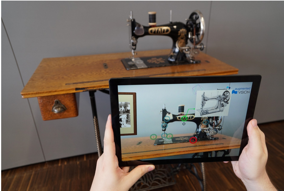
Figure 2.3.: A user using video see-through AR with an old sewing machine. By looking at the sewing machine with a tablet, the user gets additional information such as design plans, handbook, or videos showing how it was used in the past.
