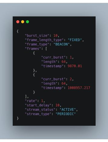
Figure 5.6: Stream log file, showing the generation of two beacon frames with a frame rate of 1 frame per second.
