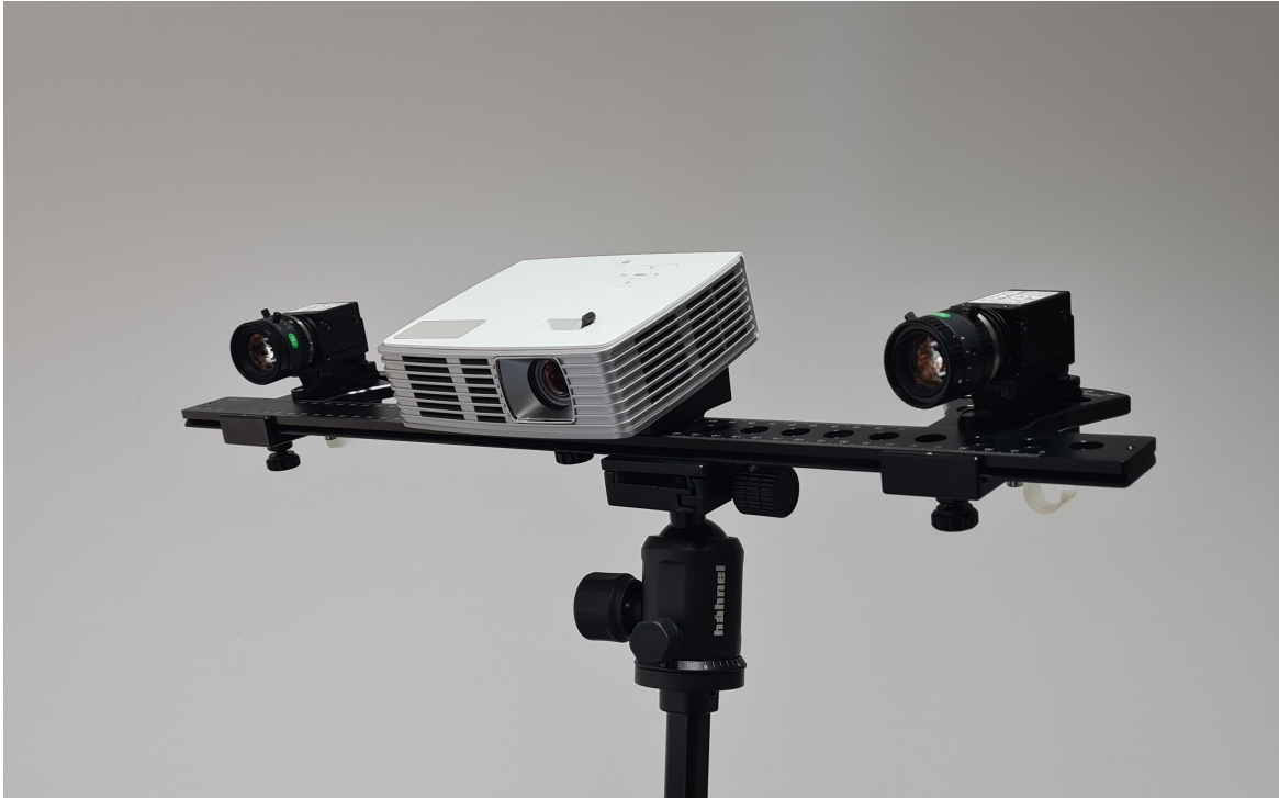
Fig. 1.11 3D-scanner: “HP 3D Structured Light Scanner PRO S3” with dual camera upgrade kit.
