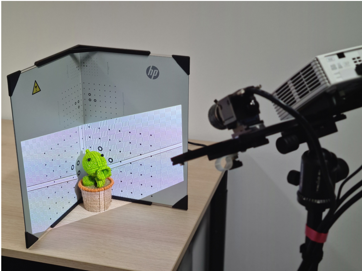
Fig. 1.12 The size of the calibration pattern is chosen according to the size of the object being scanned and the used scan window.
