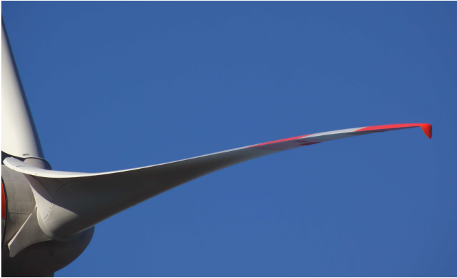
Figure 4.9. Single-blade of a wind turbine type E-101 from Enercon, detailed view of the trailing edge from hub to tip to illustrate the course of the chord length distribution and the change of the blade angle, photographer: Marc-André ABbrock
