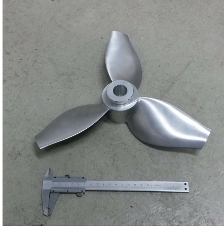
Figure 8.8. Propeller B, manufactured prototype, presentation according to Reviol et al. [182]
