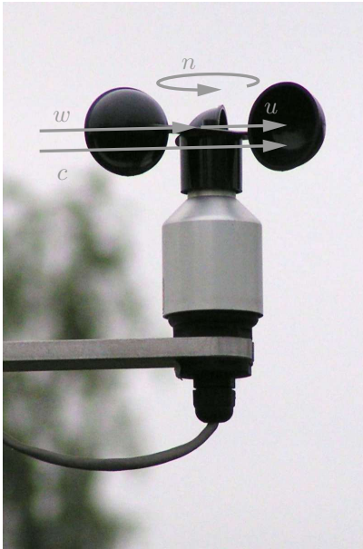
(a) Wind speed anemometer based on stagnation, Photographer: Stefan Kühn
