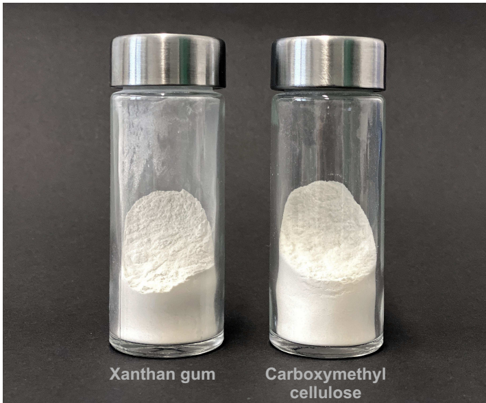
Figure 9.3. Additives used to produce the applied model fluids: xanthan gum (XG) (left) and carboxymethyl cellulose (CMC) (right), photographer: Christian Landfester
