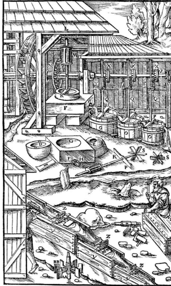
Figure 2.1. Historical application of mixers for metallurgical processes in the Late Middle Ages, taken from Kraume [121] according to Agricola [3]
