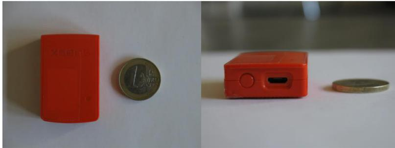
**Figure 14.** MTw Awinda MIMU (Xsens Technologies BV, Enschede, The Netherlands)
