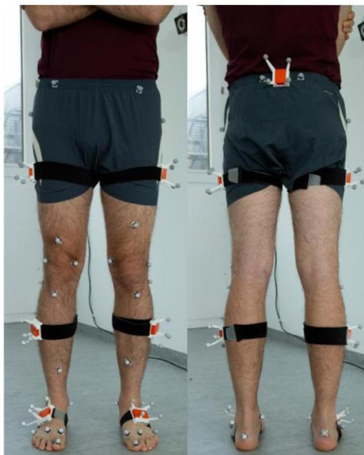
**Figure 1.** Schematic preparation of a subject with retroreflective markers and inertial measurement units (IMUs) inserted into rigid boxes equipped with additional markers. In the actual study, the markers on the pelvis were placed directly onto the skin. Furthermore, the subjects in the present study had to wear shoes.
