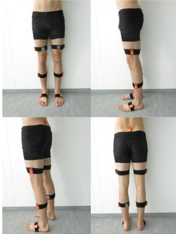
**Figure 15.** Placement of the MTw Awinda MIMUs on the segments of the lower body and the pelvis without the retroreflective markers of the OMC system.
