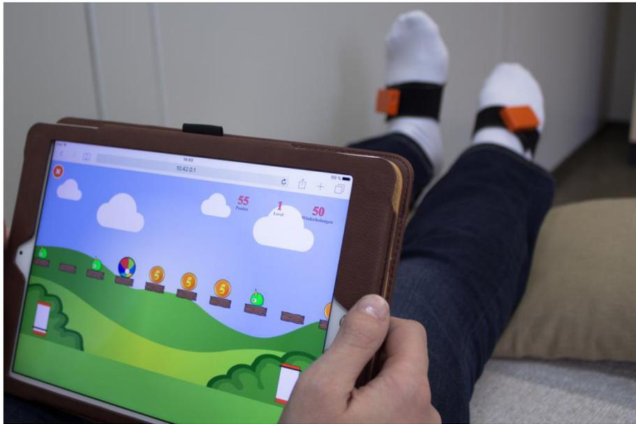
**Figure 13.** Set-up for the exergame “JumpBall”. Two MIMUs mounted on both feet are connected to an iPad (Apple, Inc.). The motion of the MIMUs triggers a jumping ball in the browser based application. Figure taken from [143].
