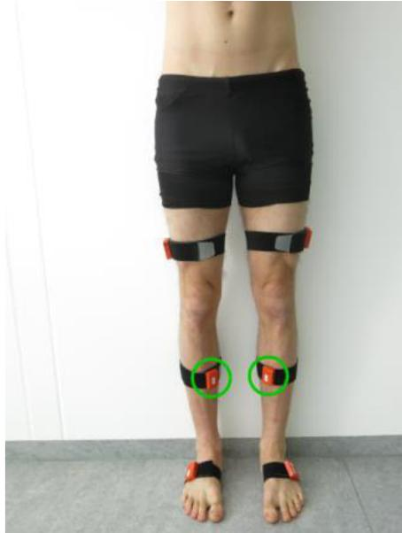
**Figure 25.** Sensor placement of the sensors assigned to the segment shank (green circle) according to official recommendations. Consider the difference in the positioning of the shank sensors in comparison to Figure 15.
