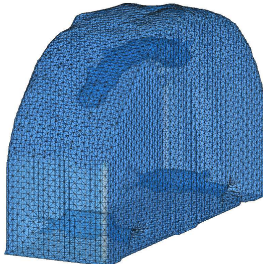
FIGURE 5.6. Transparent view of the structure after 12 iterations. The upper hole is not connected to the exterior, which means that both shape and topology optimization is performed.
