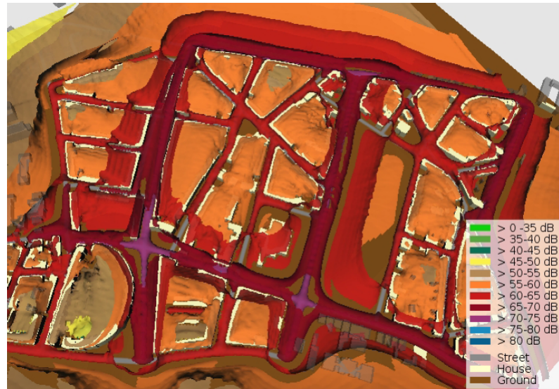
Figure 9.10: Visualization of isosurfaces every 5 dB analog to the isobands in standard noise maps.
