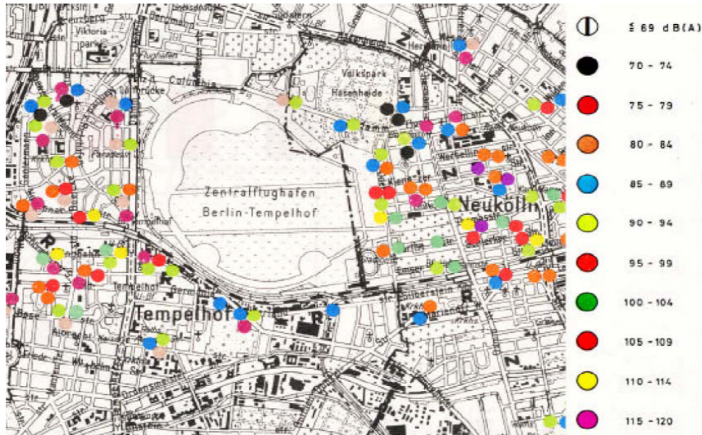
Figure 7.1: Measured air traffic noise in Berlin as colored dots on a map (1968/69) [Glü73].
