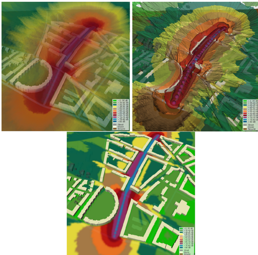
Figure 9.16: Visualization of noise emitted from a single street as volume rendering, isosurfaces and 2D noise map.
