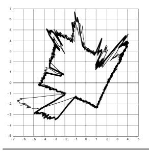
*Fig. 3* Two scans after a correction of  $43^{\circ}$  rotation, 0.14 and 0.96 m translation
