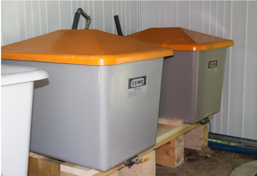
Fig. 4.10: Large volume sampling tanks used to sample the effluent (approx. 700 L)
