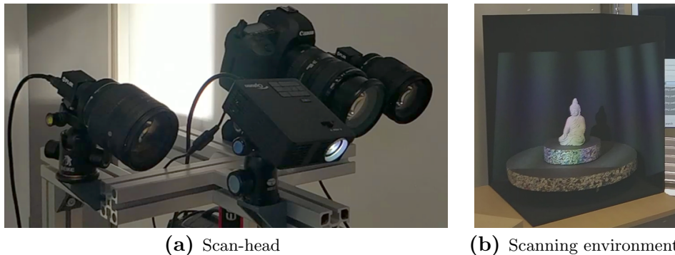
Figure 3.2.: Scan-head (a) consisting of two industrial cameras for geometry estimation, a texture camera and a video projector for scene illumination. Advantageous scanning environment (b) with turntable for comfortable rotation of the object, dark diffuse material for automatic background masking and additional texture banderole for alignment.
