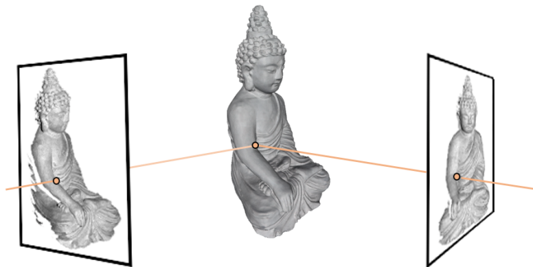
Figure 2.5.: Matching is the task of identifying corresponding image points between different views, that result from projecting the same 3D scene point to the images.
