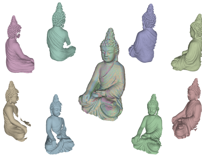
Figure 7.1.: Partial reconstructions of a full turn with 8 separate scans and the complete point cloud after alignment (middle).
