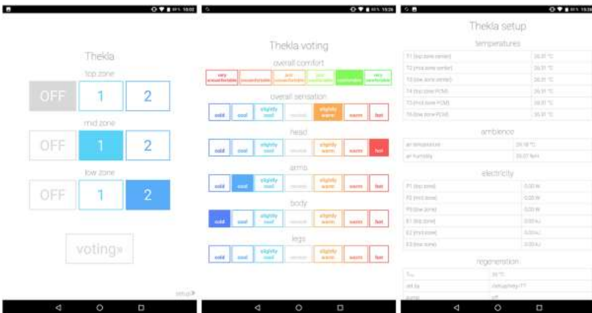
Figure 12: Screenshots of Thecla control app. Left: User front-end for control of the cooling function. Center: Excerpt of the thermal sensation voting interface. Right: Excerpt of the monitoring back-end. Own images.
