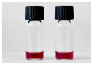
Figure S11: Images of vials containing solutions of NP R-1 (0.21 mg/mL) in water/methanol 1:2 (v/v). To the right vial Zn(NO 3 ) 2 and Na 4 P 2 O 7 were added to give concentrations of 8.3 mmol/L each. All photos were taken 5 min after preparation of the samples.
