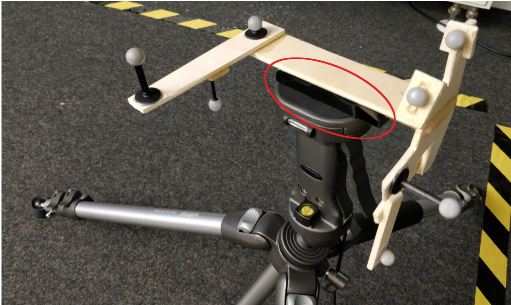
Figure 4.2: Dashboard camera with Markers Spherical markers are rigidly attached to a structure on the camera. The markers are used to form a rigid body that gets tracked by the motion capturing system (OptiTrack). Picture was taken during the data acquisition for hand-eye calibration.
