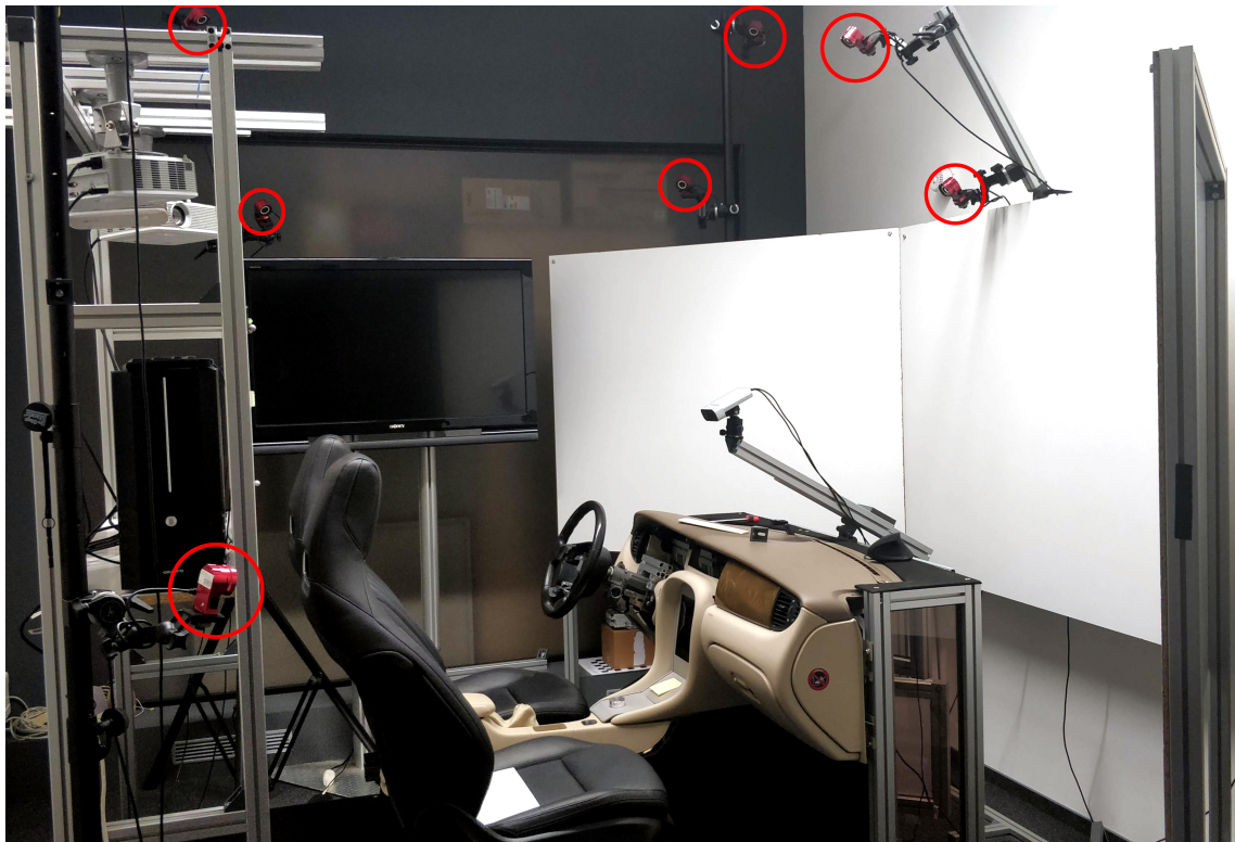
Figure 4.1: Car Cabin Simulator The red circles highlights some of the motion capture system cameras.
