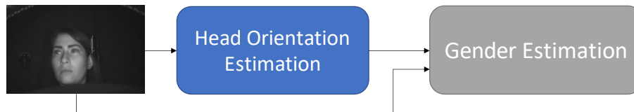
Figure 7.1: Overview. The figure depicts the abstract idea of the proposed method. First, The head image is used to predict the head orientation. Afterwards, the face image, along with the predicted head orientation angles are fed into the gender estimation model.
