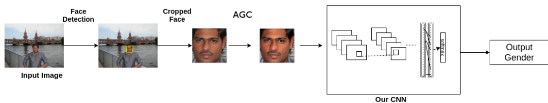
Figure 6.9: Gender Recognition Pipeline for Still Images. The pipeline starts with an input image. The image is processed and the face is detected. Afterwards, the face image is cropped and then the face image is enhanced using AGC. The enhanced face image is fed to the GenderCNN for predicting the gender from the image, and outputs the predicted gender.
