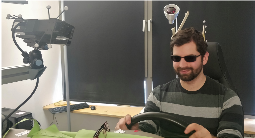
Figure 4.3: Center mirror camera with markers. Spherical markers are rigidly attached to a structure on the camera (Kinect v2). The markers are used to form a rigid body that gets tracked by the motion capturing system (OptiTrack). Also a subject is shown wearing sunglasses and the head target with markers to be tracked by the OptiTrack.
