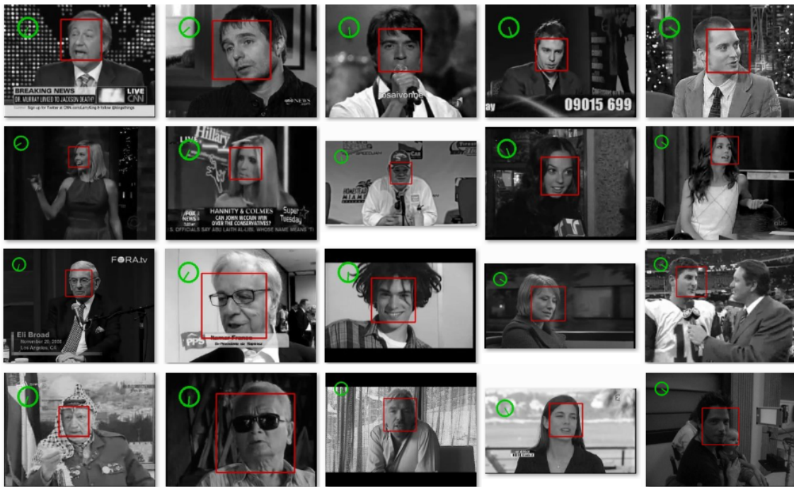
Figure 3.1: Samples: Yaw angle estimation on YouTube face dataset. The red rectangle depicts the detected face, and the estimated yaw angle is indicated inside the green circle at the top-left corner. The circle represents a top view of the face, and the green line inside it shows the detected yaw angle. A detected angle of 0^\circ is indicated by a line pointing downward. Despite the images having different backgrounds, presence of eye glasses or not, or some occlusion on the face, our method can predict the head orientation correctly
