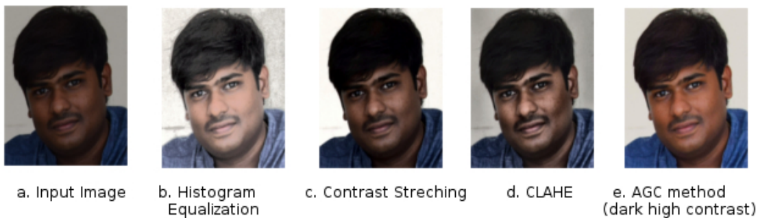
Figure 6.3: Image Enhancement Techniques. (a) Input Image. (b) Histogram Equalization: result is over or under-enhanced regions. (c) Contrast Stretching. (d) CLAHE. (e) Adaptive Gamma Correction - AGC.
