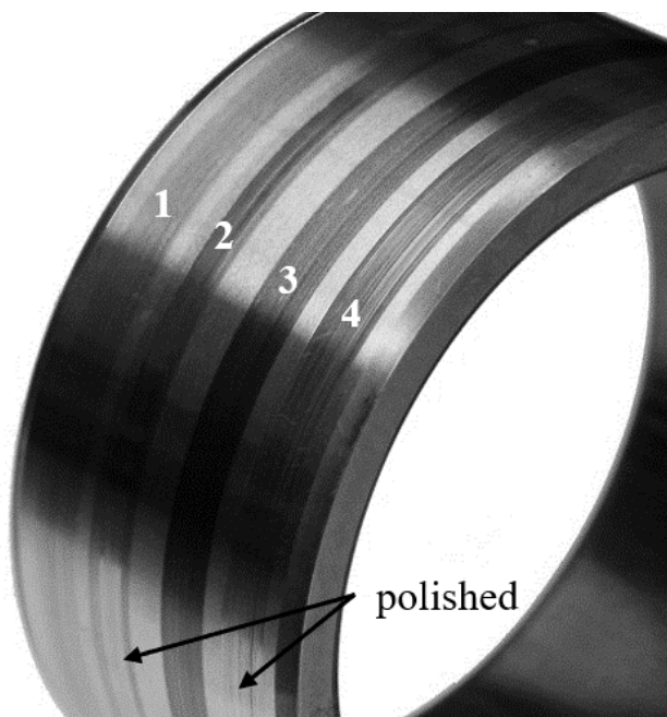
Figure 42: Example of local increase or decrease of brightness due to polishing, depending on angle, camera position and ring curvature.
